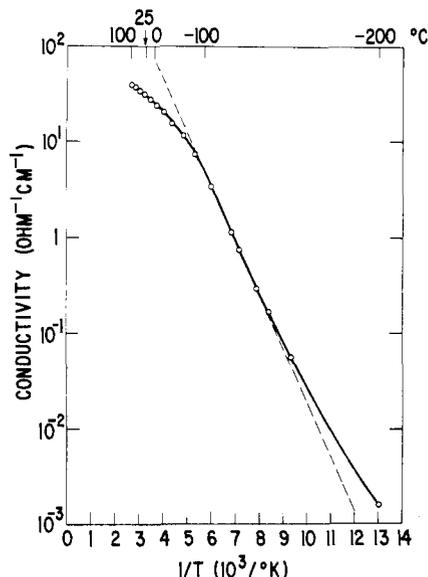
**Figure 2.** Conductivity ( $\sigma$ ) of a  $\text{TTT}_{1.2}\text{NiS}_4\text{C}_4\text{H}_4$  crystal as a function of temperature. The dashed line, which indicates the region of maximum slope of  $\log \sigma$  vs.  $1/T$ , is drawn to illustrate the nonlinear character of the  $\log \sigma$  vs.  $1/T$  dependence.
